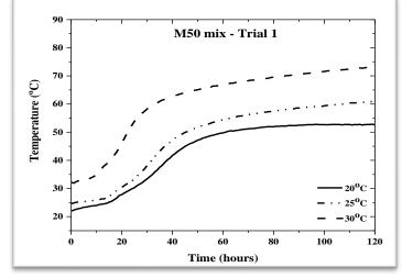
Temperature profile of concrete placed at different temperatures
